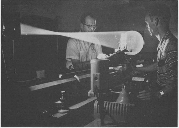
CONE OF LIGHT inside the optical development lab is shown in this photograph. Bright rectangle near the mirror is a solar cell undergoing test with
